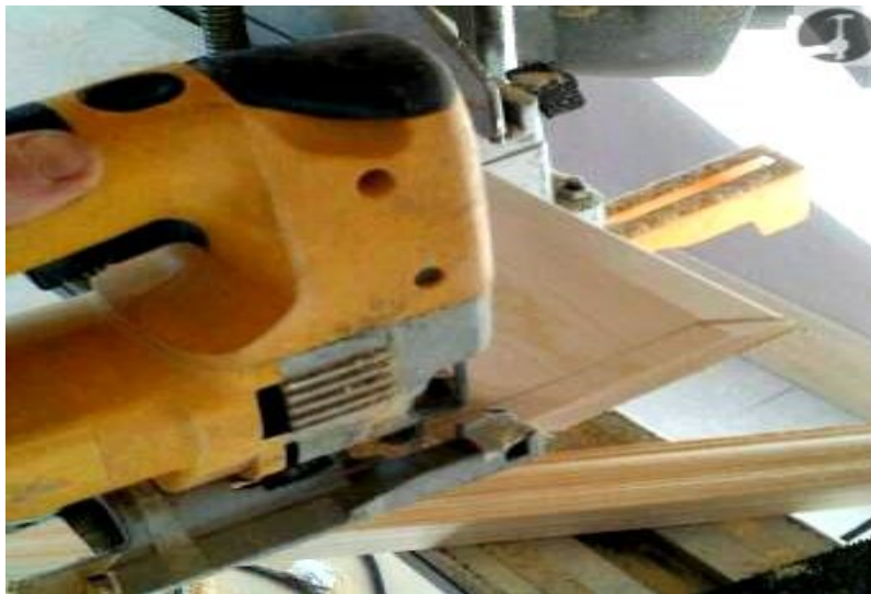
Figure 11 cutting with jigsaw
